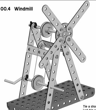
Tie a short piece of string into a loop just big enough to fit over the two pulleys tightly, and then the handle at the bottom will turn the sails.
