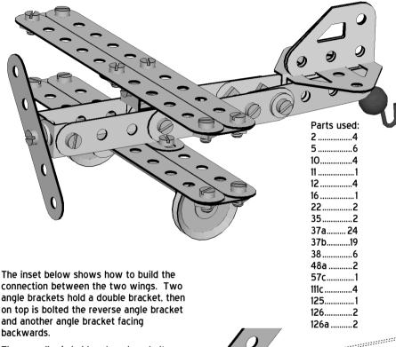
The propeller is held on by a long bolt, which holds the propeller first, then a nut, then a washer, then the angle bracket and double angle strip (the far side of the fuselage), and finally another nut. The two nuts are tightened against each other, leaving the propeller to run freely.
