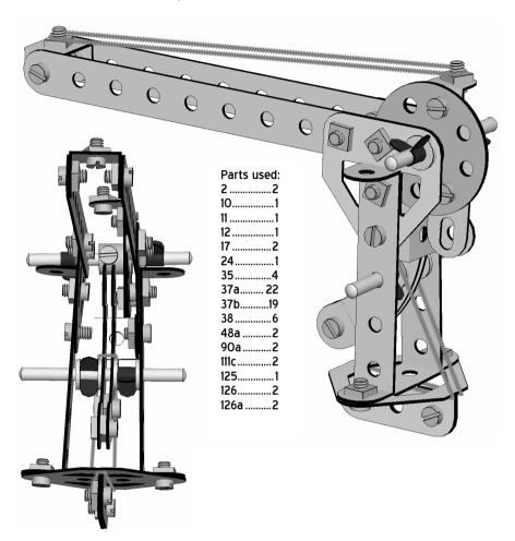
Begin by building the complete framework of strips, double angle strips, trunnions, and flat trunnions. Notice the reverse angle bracket bolted to the left-hand side, pointing backwards.
