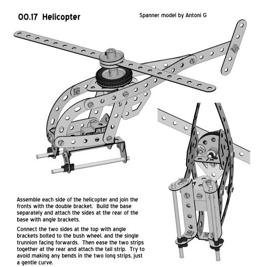
The tail rotor in this illustration is held by a long bolt (part 111c), with a nut securing it to the tail, then a washer and the rotor with two nuts lock-nutting the rotor to the tail. There are various ways of lock-nutting this part on.
