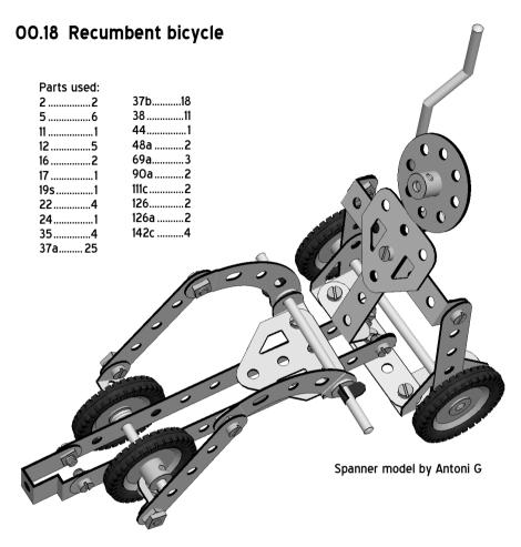
The base of the bicycle consists of the two  $5\frac{1}{2}$ " Perforated Strips connected together at the rear by the Double Bracket. This Double Bracket is lock-nutted to the  $2\frac{1}{2}$ " strip, from which the rear of the bicycle and the rider's body is built.
