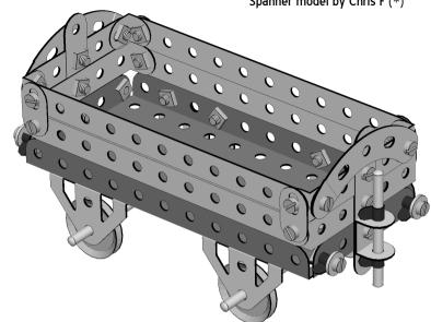
This model uses all the nuts in the outfit, and even then three of the trunnions used to support the wheels can only have one nut and bolt each (they would be better with two, as shown in the picture to the right).
