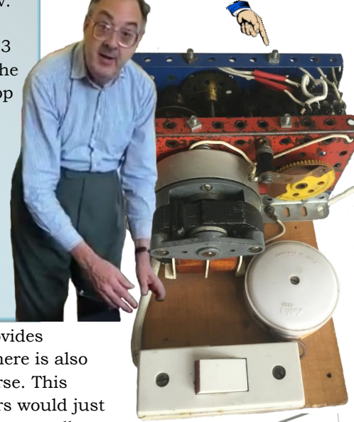
Auto Timer with a Crouzet motor and half-on/half-off commutator.
