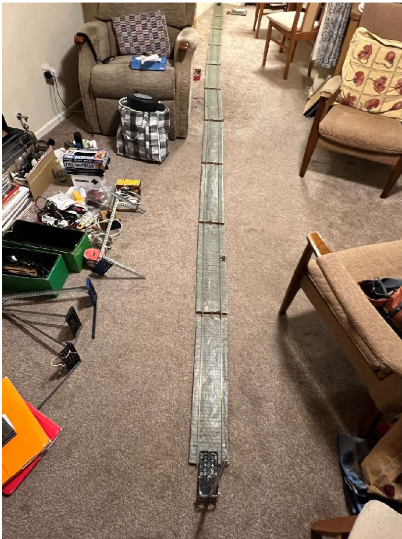
One of the green boxes has thick card rectangular pieces in it, as well as folded V-shaped cards. The flat sections can be placed under the ends of a given track length should vertical adjustments be required to keep the track horizontal.
